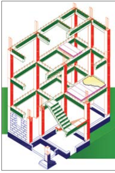
Fig.1: Structural configuration of 3S System
